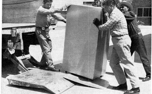
RUDY LUCERO, left, demonstrates how an aluminium plate attached directly to the power tail gate of the devilery truck simplifies the loading job. The heavy safe can be rolled directly onto the gate, impossible to do without the plate. It saves about four minutes per job. At right are Manuel Sanchez and Fidel Gonzales.
